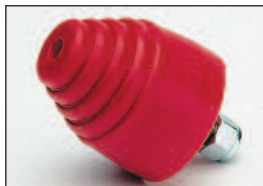
9.9101 All purpose bump stop for control arms, traction bars & leaf springs. Designed to be easily trimmed for custom fit. 2 1 / 8 " tall, 2" dia. 2 per set.
